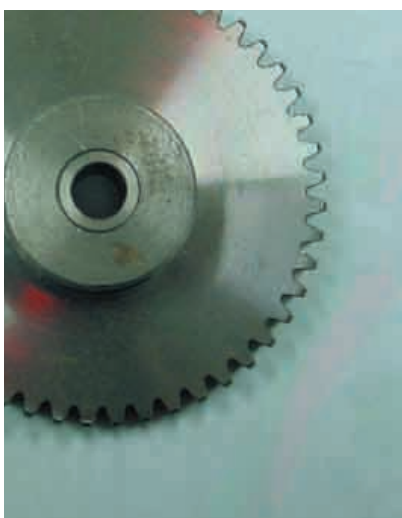
Polewheels and polebands used in rotating machines to detect speed information
